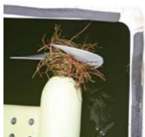
Hatches in the cockpit sole make it easy to clear a prop wrap
