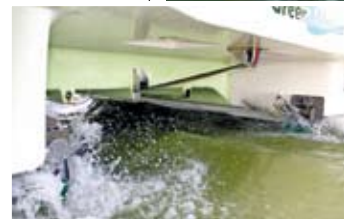
The motorgen saildrives lift, reducing drag while sailing and galvanic corrosion while moored
