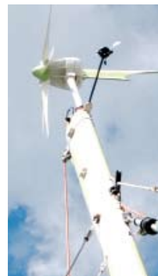
Mast-mounting the D400 wind generator improved its output by a factor of 2.4
