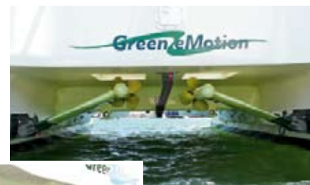
The motorgen saildrives lift, reducing drag while sailing and galvanic corrosion while moored
