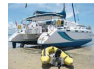
African Cats are designed to dry out on keel stub and rudders
