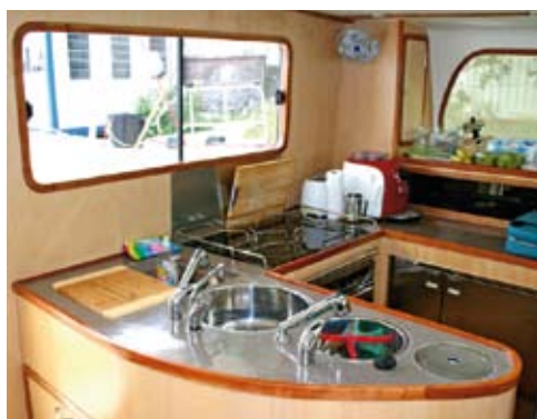
The power-hungry galley has an electric oven and hob, a fridge and freezer, boiling water on tap for drinks, an espresso machine and a dishwasher
