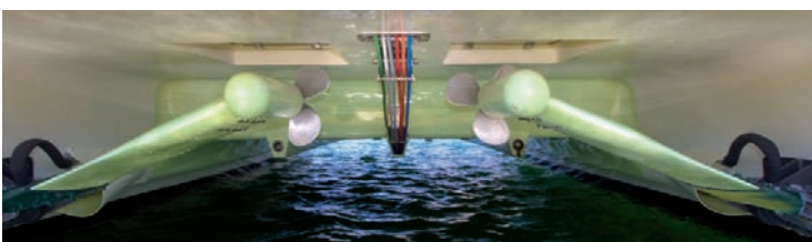
The famous 'Motogens' which retract to avoid drag, once the batteries are charged.
